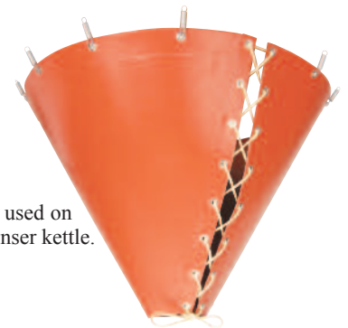
Formed heater with six thermocouples for six-zone control used to refurbish airplane propellers by applying heat to cure an epoxy compound that attaches a new nickel lead edge to the propeller blade.
